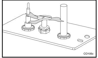
Fig. 51 Correct pilot flame pattern. SIT pilot.
